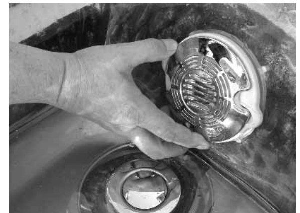
Replace screen by turning clockwise
