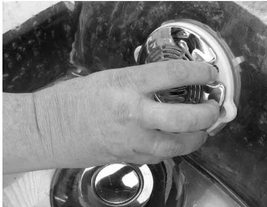
Remove screen by turning counter-clockwise.
