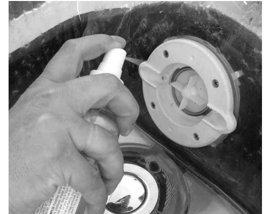
Clean intake area using a soft bristled brush or cloth and low foam soap to remove any visible residue. Rinse with sprayhead - Cold water
