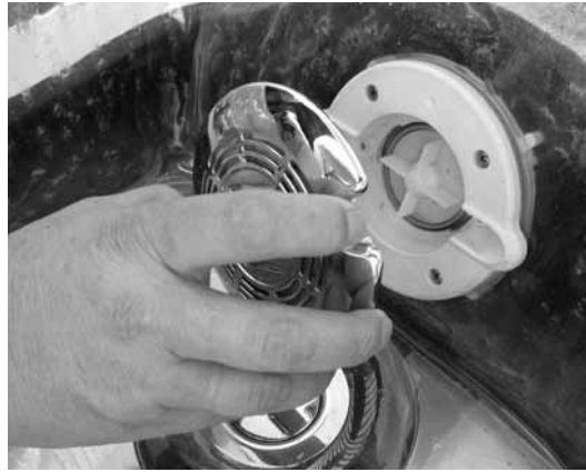
Clean intake area using a soft bristled brush or cloth and low foam soap to remove any visible residue. Rinse with sprayhead - Cold water
